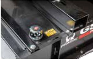
Integrated metal fuel tank
